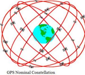
4 Satellites in 6 Orbital Planes 4 Satellites in each plane 20,200 km Altitutes, 55 Degree Inclination
